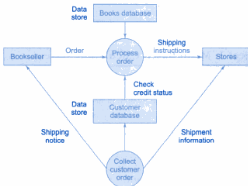
Fig. 17.16 ⇔ Data flow diagram for order processing and shipping for a publishing company
